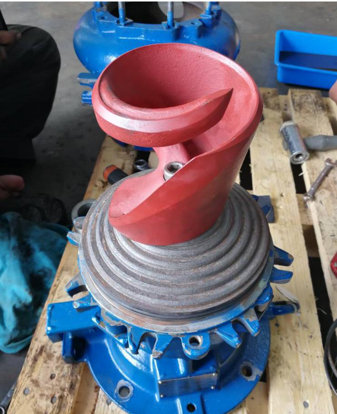
Pump Impeller replaced
