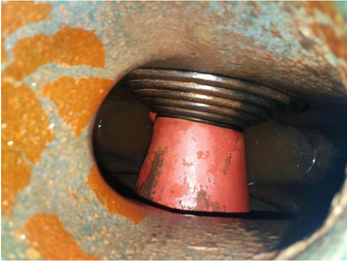
Pump passed leak tests under pressurized condition ( gasket sits perfectly ) - Flow test passed
