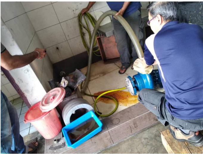
Pump passed leak tests under pressurized condition ( gasket sits perfectly ) - Flow test passed
