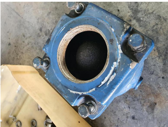
Vacuum pump oil completely emulsified with water and sewage , not usable
