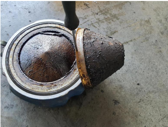
Exhaust valve jammed and the body rusted, damaged due to moisture Installing external strainer is mandatory
