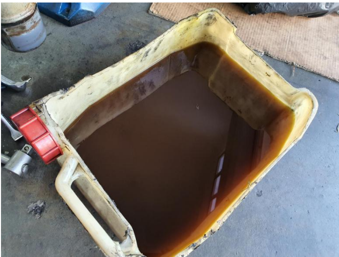
Vacuum pump oil completely emulsified with water and sewage , not usable
