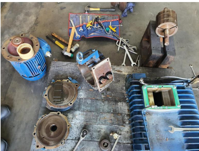
All parts will be chemical washed to ensure no debris and particles attached onto the metal surface
