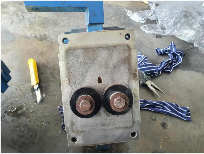
New Exhaust valve installed and base polished
