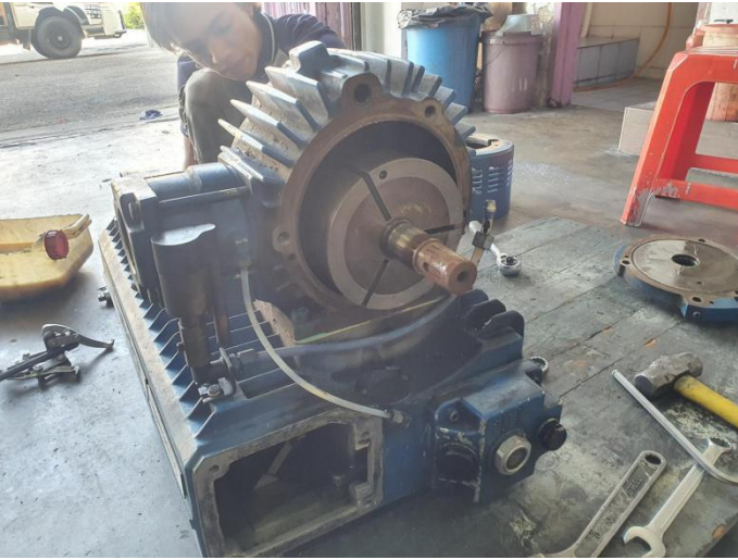
Pump vanes badly damaged , impossible to build pressure
