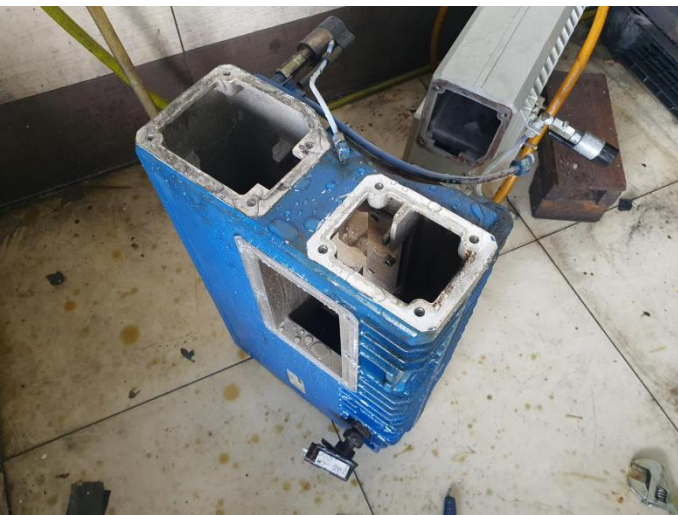
Pump Module chemically washed
