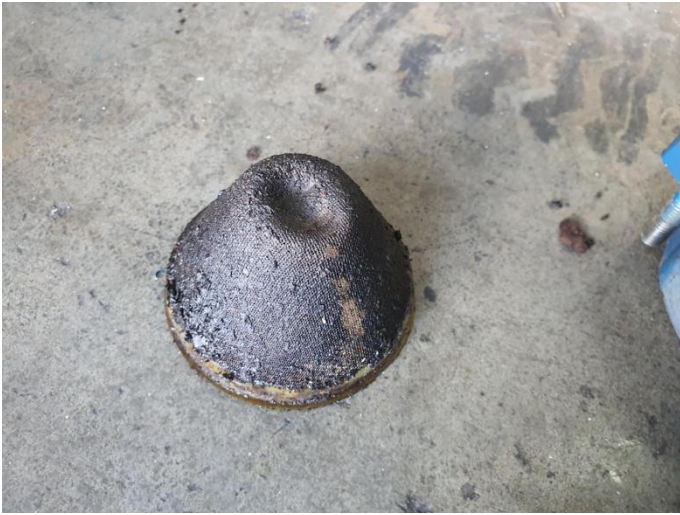
Pump internal strainer choked with dust, debris, sewage and moisture Installing external strainer is mandatory
