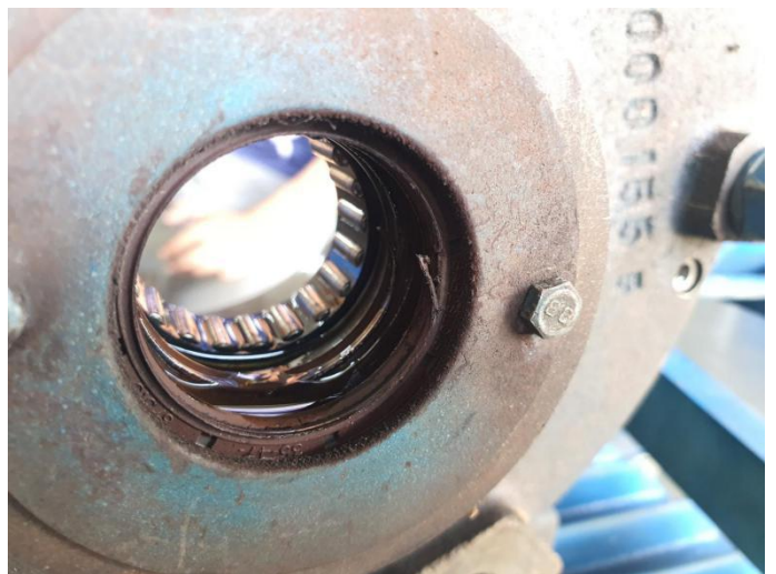
Bearing seal damaged, Vacuum pump oil will always need to top up as it will flow out in exhaust line
