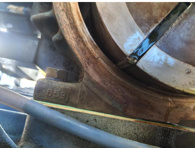
Bearing seal damaged, Vacuum pump oil will always need to top up as it will flow out in exhaust line
