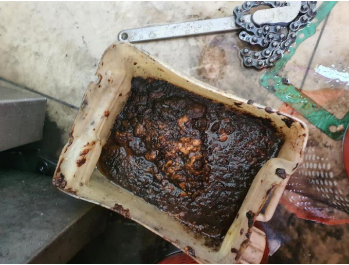
Sludge removed from pump
