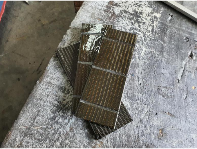
Vanes damaged , rotor requires polishing
