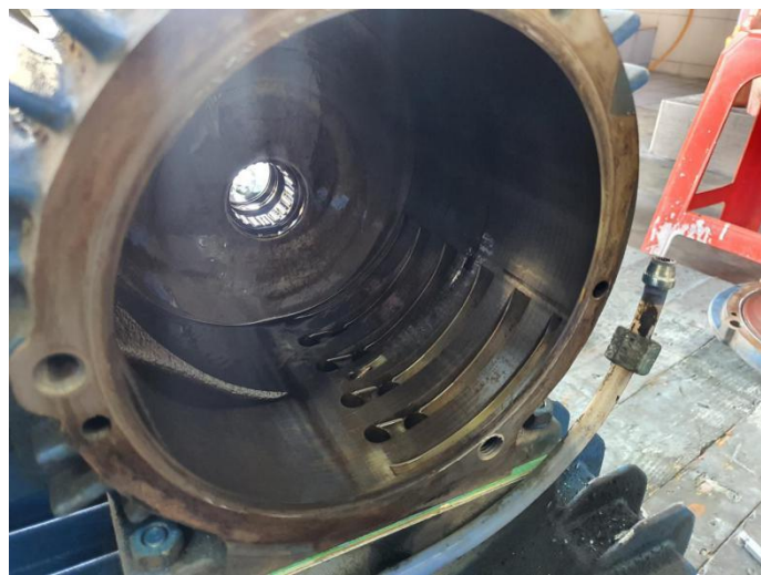
Cylinder worn out , requires polishing to reduce friction upon running
