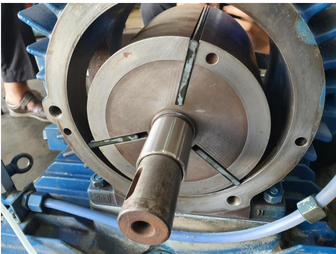
New Vanes installed ( Original )
