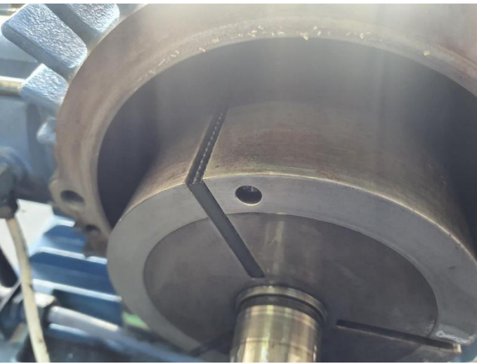
Pump vanes badly damaged , impossible to build pressure
