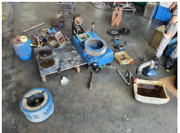
All parts will be chemical washed to ensure no debris and particles attached onto the metal surface
