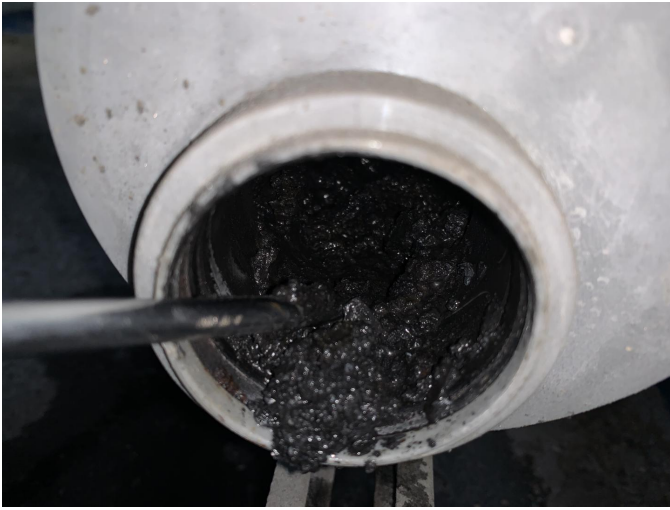
We noticed a piled up debris in the exhaust line
